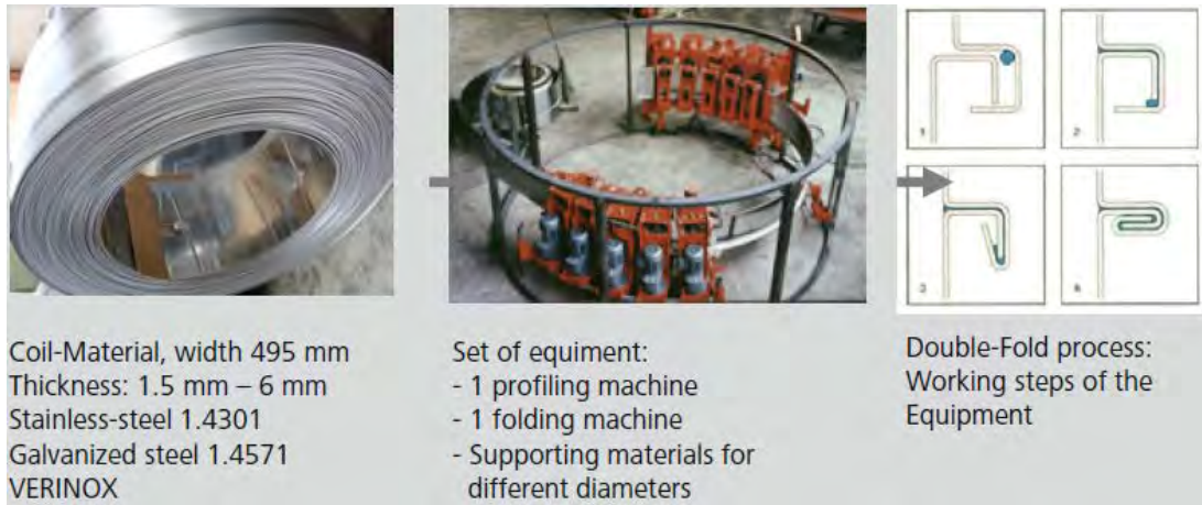
Figure 2: Verinox coils composition, geometry and assembly
